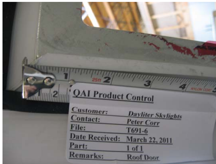
Fig. 8 – Corner of aluminum reinforcement frame
