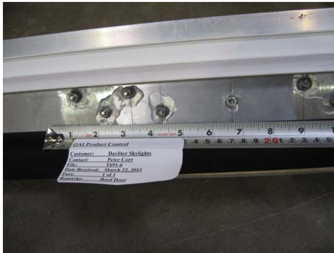
Fig. 5 – Aluminum sash stiffener fastener and hinge screws
