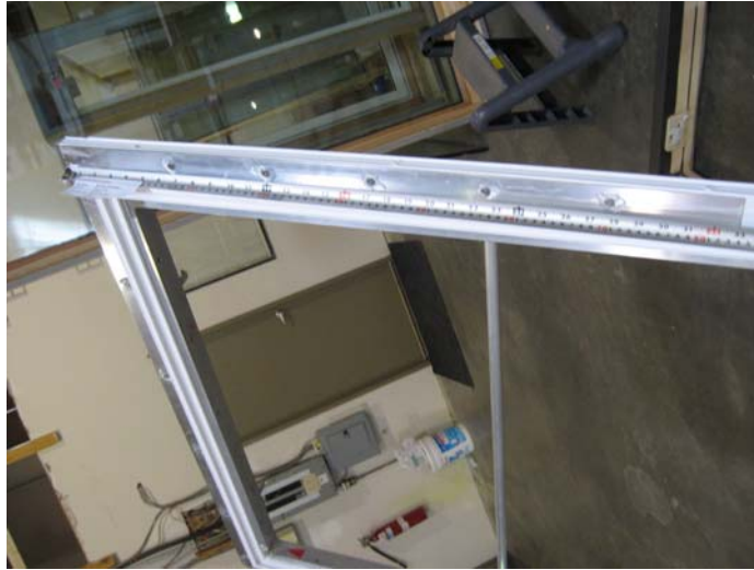
Fig. 4 – Aluminum sash stiffener
