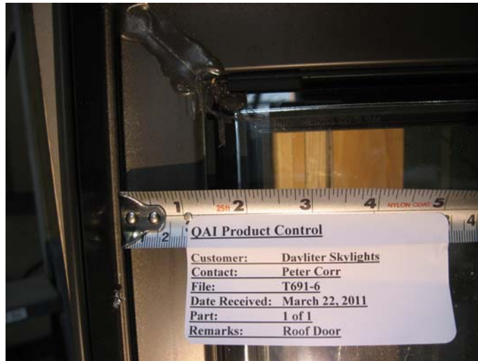
Fig. 2 – Aluminum cap corner joint seam sealer and setting blocks
