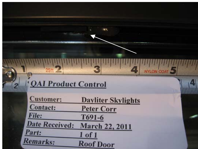
Fig. 3 – Setting block along length of sash
