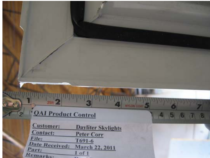
Fig. 7 – Corners of sash trimmed
